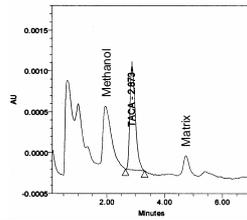
Fig. 4 Chromatogram of a tape with skin, spiked with TACA solution (0.75 µg TACA /tape).
